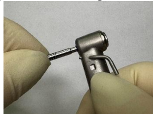
2.Insert the key into the contra angle until you hear a "click"
