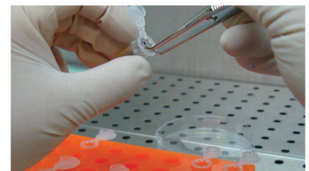
Fig. 2. A Cone Morse taper internal connection placed into nutrient solution.
