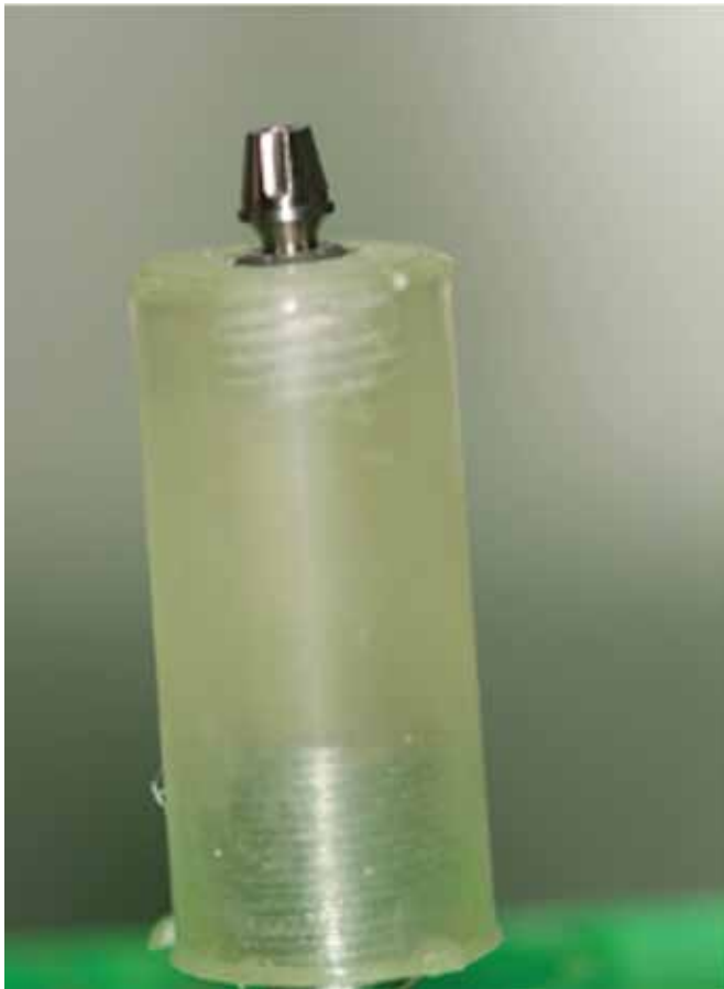
Fig. 1 - Abutment connected to the implant at 30 N cm.
