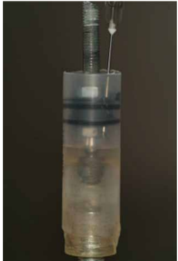
Fig. 2 - Implant/abutment immersed in nutrient solution, drawn by sterile syringe and analyzed by culture method.
