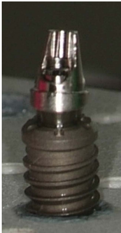
Fig. 1. An assembled implant-abutment after inoculation with a bacterial suspension.
