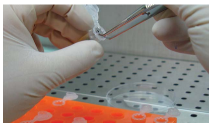
Fig. 2. A Cone Morse taper internal connection placed into nutrient solution.
