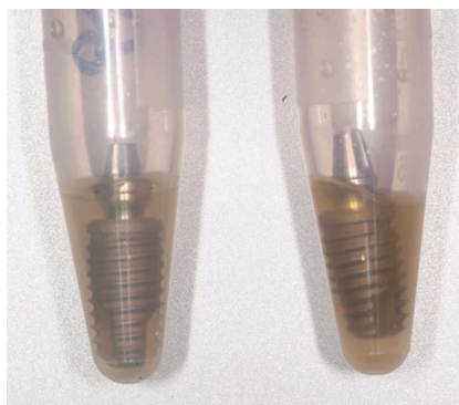
Fig. 3. Left: no contamination. Right: turbidity of the broth as a sign of bacterial penetration.
