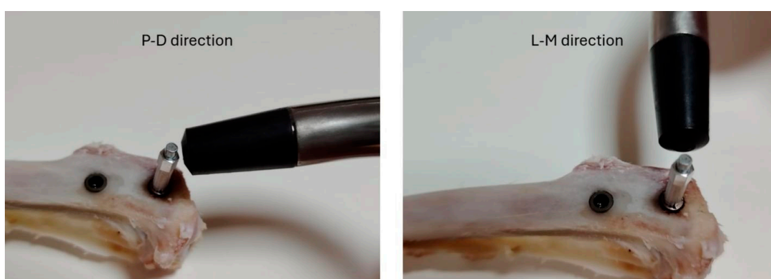
Figure 5. Measurements of the implant stability using the Osstell system in two directions (proximodistal (P-D) and lateromedial (L-M)).
