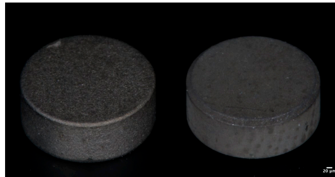
Figure 1. Representative image of the disks used: (left) surface treated with \text{TiO}_2 sandblasting; (right) surface treated with combined treatment \text{TiO}_2 and HCl.
